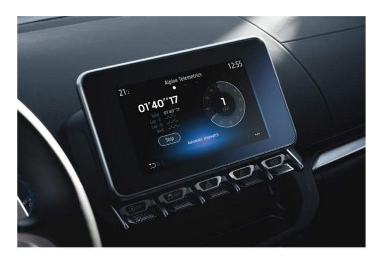
Alpine Telemetrics provides real-time access to technical data recorded by the vehicle's sensors (pressures, temperatures, engine speed, steering wheel angle, etc.) and presents it via digital graphs. In addition, the integrated chronograph allows you to measure lap timing and performance.
