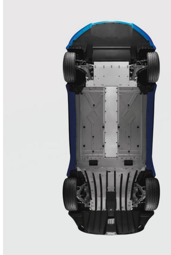
Alpine engineers have also paid particular attention to the aerodynamic development of the Alpine A110, using technical solutions borrowed from the world of racing. Thus, the A110 features an integral flat floor, a technique carried over from the world of high-level motor racing. Thanks to a rear diffuser located beneath the rear bumper, the A110 offers excellent rear handling.
