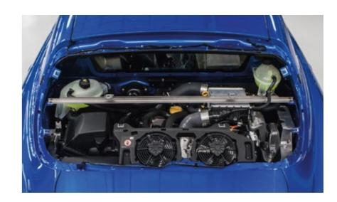
Tuned by Alpine powertrain engineers, the 1.8-litre direct injection engine delivers thrills and strong performance. The new 300 hp engine offers a torque of 340 Nm generously available from 2,400 to 6,000 rpm, accelerating (A110 R version) from 0 to 100 km/h in 3.9 seconds and reaching up to 285 km/h on track.
